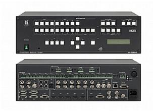
The VP-725NA is a presentation scaler/switcher with multiple signal format sections and balanced stereo audio. The unit has five independent 4x1 video sections: composite, s-Video (Y/C), component (YUV), computer graphics and HDMI, plus a single USB input. It also scales any video input up or down to a selectable graphics or HDTV output resolution and provides glitch-free switching between sources through FTB<sup>™</sup> (fade-thru-black) switching technology.
