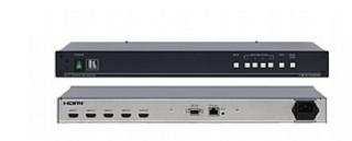
The VS-41H is a high-performance switcher for HDMI signals. It reclocks and equalizes the signal and switches one of the four inputs to a single HDMI output.
